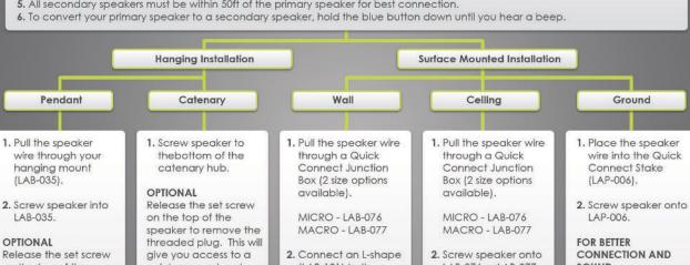
on the top of the speaker to remove the threaded plug. This will give you access to a quick connect port. This allows for a light fixture to be attached to the speaker.
